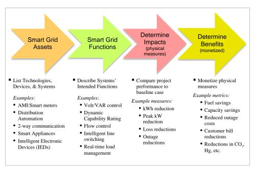
Figure 5-1 Conceptual Overview of the Smart Grid Evaluation Process
